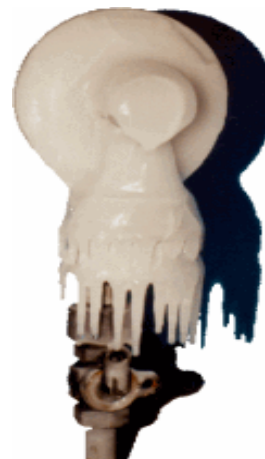
Freeze test photo of Vent Skirt installed on Service Riser regulator
