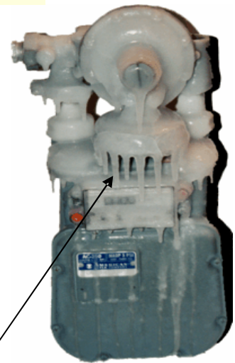
Freeze test photo of the MBVS-1200 Vent Skirt installed on Meter Bar regulator
